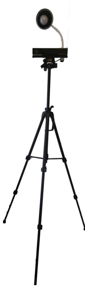
Figure 9: Kinect mounted on tripod set at height of 160 cm. Additional light source was added to the top of the Kinect allowing for consistent lighting during each acquisition.
